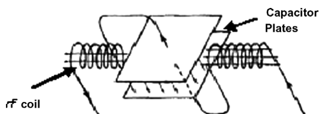
Fig. 5. A schematic diagram of the “Slepian” drive [99].
